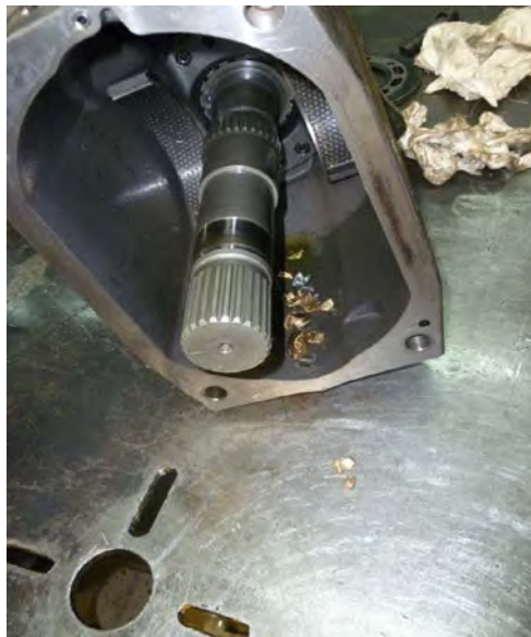
Figure 6-5. Cavitation Damage on a Hydraulic Pump.
