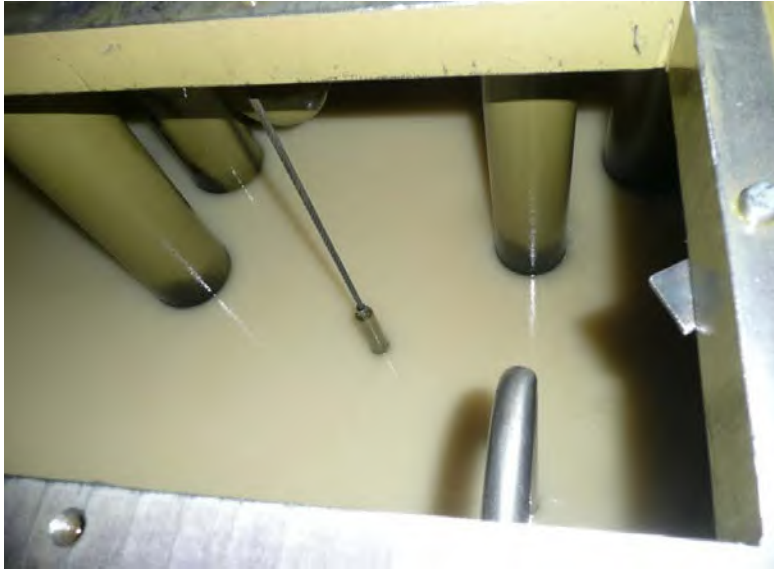
Figure 7-7. Extreme Foaming in the Sump of a System in which ASTM D892 Antifoaming Properties Were Not Adequate.
